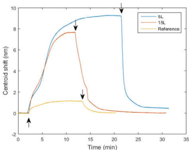
**Figur 2. Centroid shift as a function of time and HKUST-1 layer thickness. The first arrow marks the introduction of cyclohexane into the system. The following arrows marks the switch to pure argon.**
