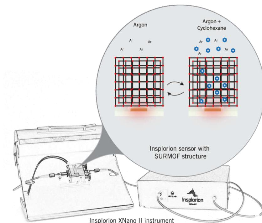
**Figure 1. Insplorion sensors functionalized with a SURMOF. The metal-organic framework has the ability to host large amounts of guest molecules, in this case cyclohexane.**
